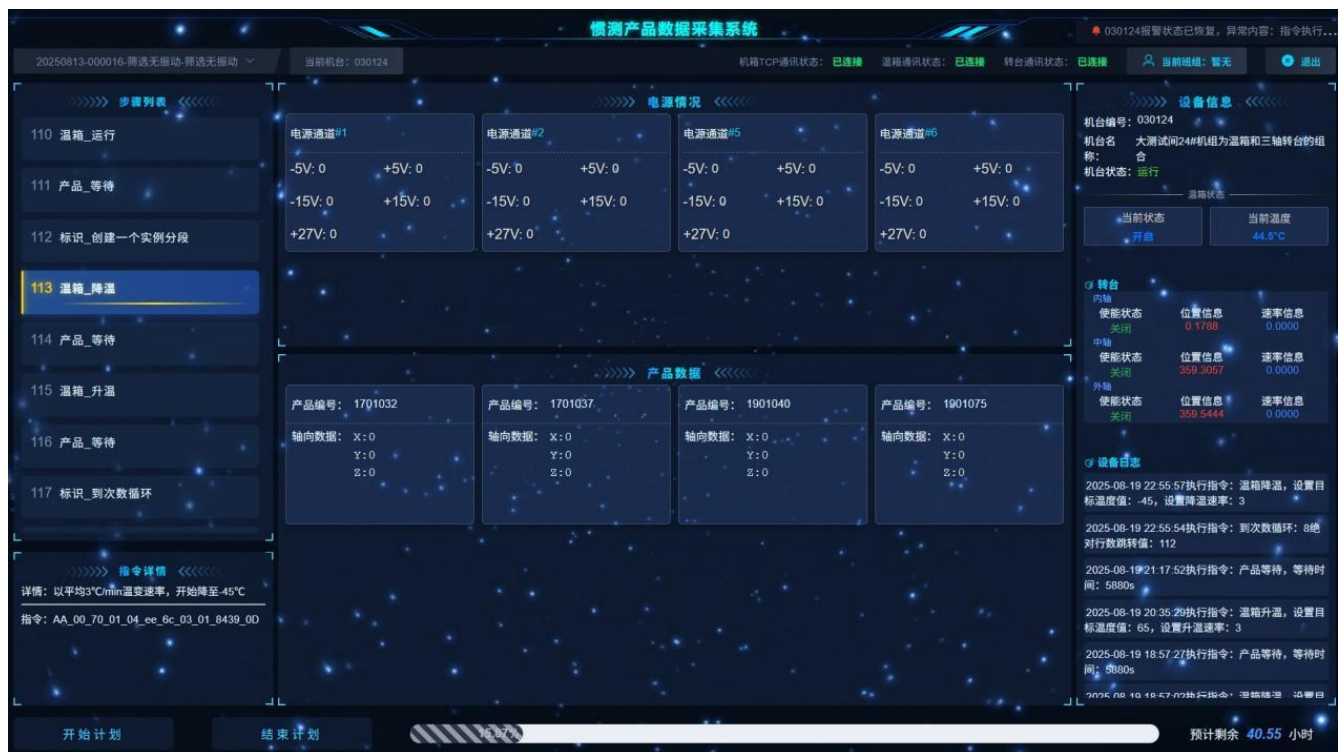
Figure 2 Data Acquisition System for Inertial Measurement Products
